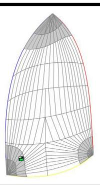
Computer designed and cut tri-radial construction using Contender Superkote 75 (100%) [Panel Diagram: Renegade Asy 3 Seam 11]
